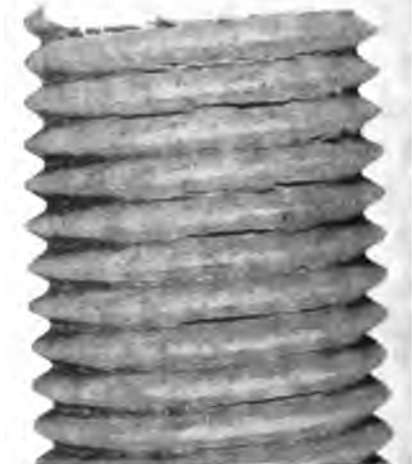
Fig. 3. Incipient Cracks at Base of Threads.†
